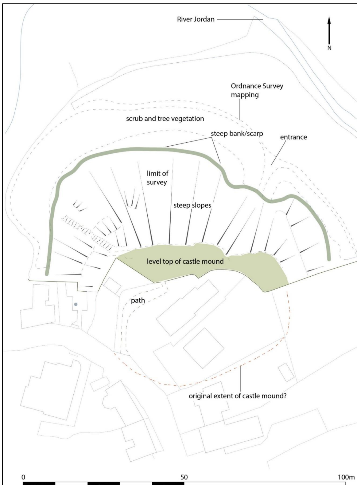
Fig 7 Bottreaux Castle 2021 Total Station Survey.
